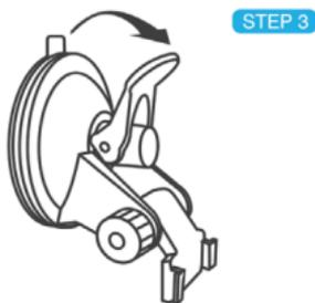
Ensure the locking lever is in the UP position.
